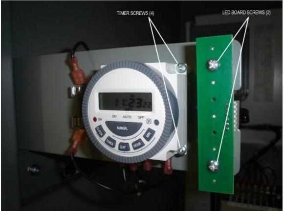
Figure 6. TIMER AND LED BOARD MOUNTING
