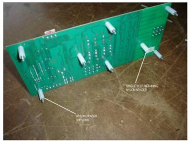
Figure 3. CONTROL BOARD NYLON SPACERS
