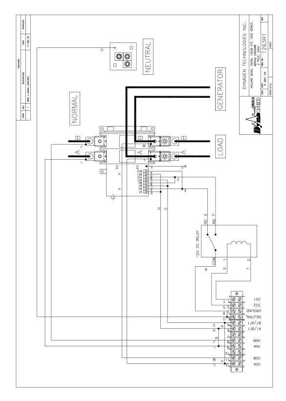
8:10 VTS1-0600-2-240-12 WIRING DIAGRAM
