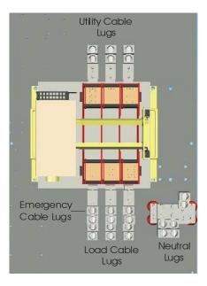
**WARNING:** 600A models include factory installed protective shields covering the power connections of the switch mechanism. Be certain to reinstall the supplied transparent protective shields to the switch mechanism after the proper connections are performed.
