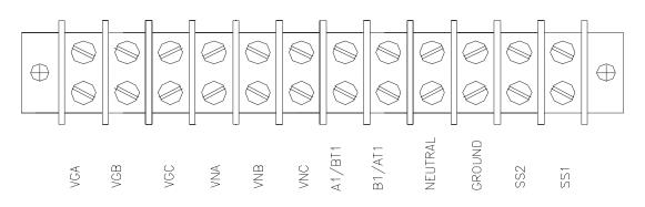
\* Please note the VTS1000 Series Transfer Switch consists of the above 12 position terminal block for customer sensing connections. See wiring diagram for sensing positions.
