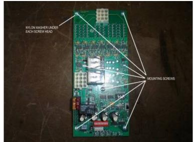
Figure 2. CONTROL BOARD MOUNTING SCREW LOCATIONS
